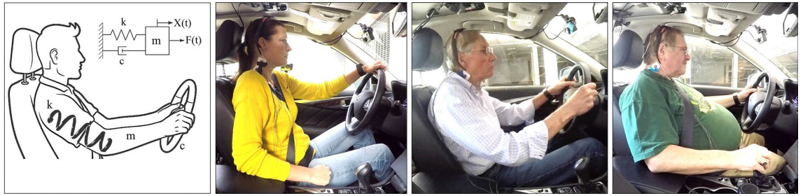
Figure 1. Individualized driver stress detection method using an unmodified car steering wheel.
