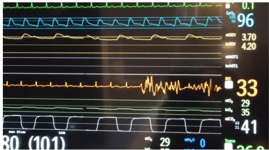
FIGURE 1: EKG signal being picked up on BIS monitor (orange waveform, numerical value 33)
