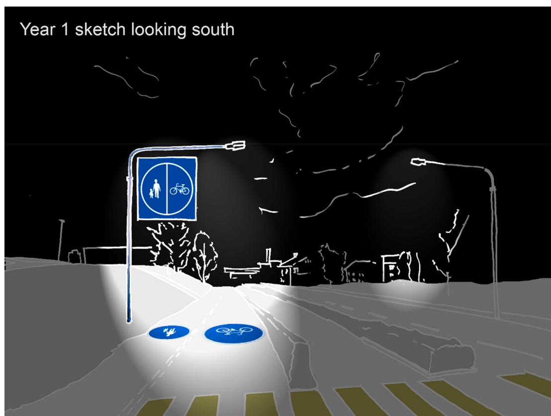
Figure 8. An illustration of seasonal winter cycle lanes that are being tested by Lulea University of Technology in Kiruna, Sweden. Here winter cycle lanes are marked out using projected information on to the snow and ice and separated from vehicular traffic by low snow walls (copyright: David Chapman).
