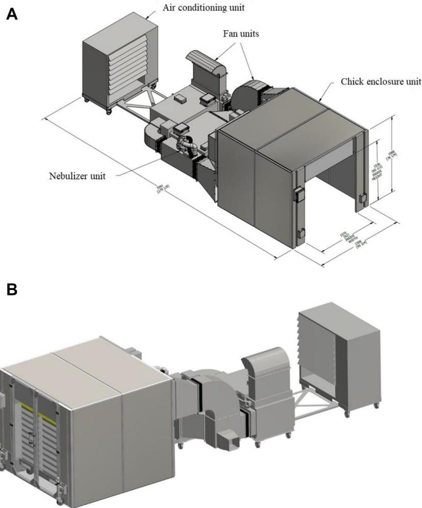
**Figure 1.** Conceptual design of the CSPN (commercial-scale poultry nebulizer). (A) Left view of the CSPN, and (B) right view of the CSPN.
