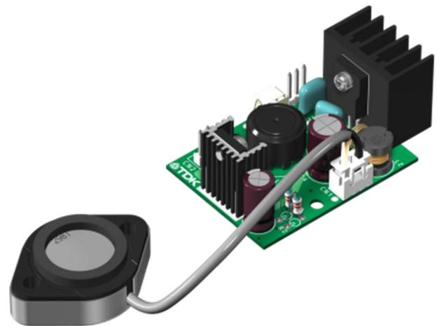
**Figure 2.** Ultrasonic-type nebulizer. An individual ultrasonic type nebulizer that consisted of a piezoelectric ceramic plate with the ability to generate high-frequency ultrasonic waves to convert the CpG-ODN solution into aerosol droplets. An array of these was used. Abbreviation: CpG-ODN, cytosine phosphodiester guanine oligodeoxynucleotide.
