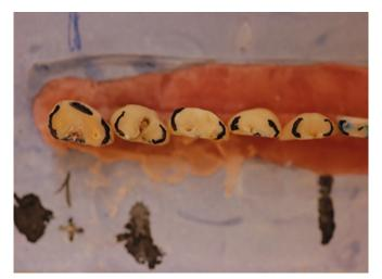
Fig. 1: "Teeth" mounted on a hard plaster stand base before grinding procedure
