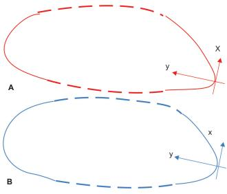
Figs 3A and B: Tooth contour before and after grinding procedure. The local (x, y) axes are shown
