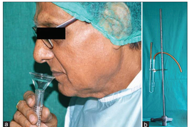
Figure 1: (a) Collection of saliva by spitting method (b) Ostwald viscometer tube with stand
