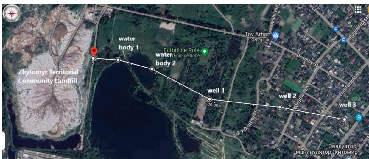
Fig. 3. Scheme of water sampling from surface water bodies (Distance from the landfill boundary: water body 1–100 m, water body 2–250 m) and wells (Distance from the landfill boundary: well 1–500 m, well 2–750 m, well 3–1000 m) materials from the site https://www.google.com/maps ; coordinates: latitude – 50.30316, longitude – 28.64262, Scale 1:5000.
