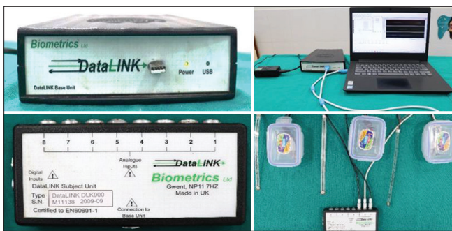
Figure 1: DataLINK Software and Hardware Biometrics Ltd data acquisition unit and its connections
