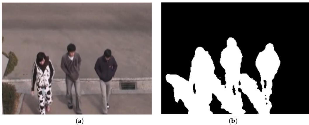
Figure 2. Foreground region extracted in a video content analytics algorithm: (a) Input video frame; (b) Foreground region extracted.
