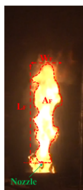
Figure 4. Flame geometry features of jet fires.
