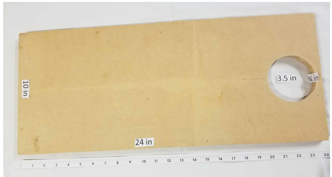
FIGURE 4: MDF board component of the pelvic model
