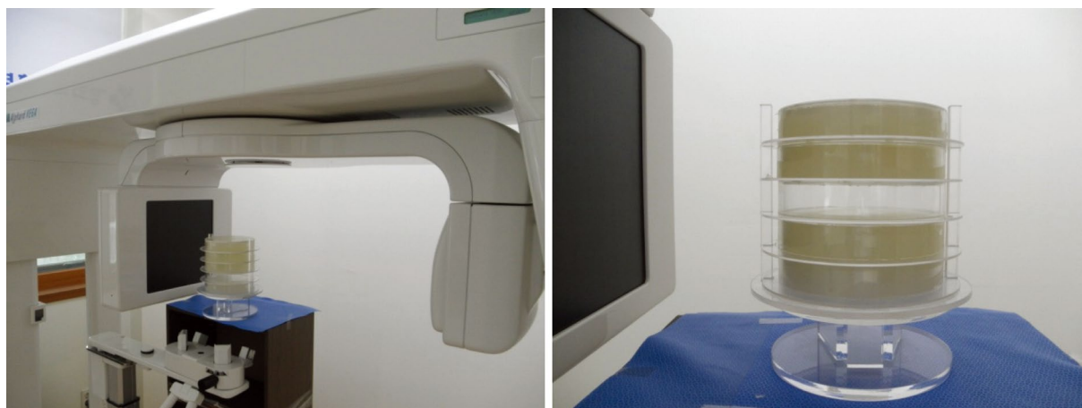
Fig. 2. Four geometric reference objects were placed in the cylinder assembly and scanned in the cone-beam computed tomography device.
