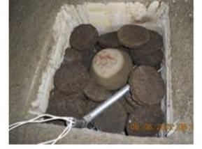
Fig. 1. Partly filled Varaha Puta with cow dung cakes
