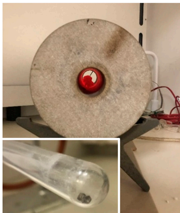
Figure 7. The thermal treatment, the tube furnace glowing at 650 °C, and the magnification of the diamonds post-treatment in a quartz glass tube.
