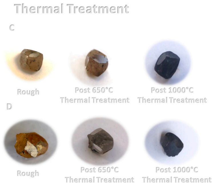
Figure 8. Daylight photographs of the pre- and post-thermal treatment of diamonds C and D.
