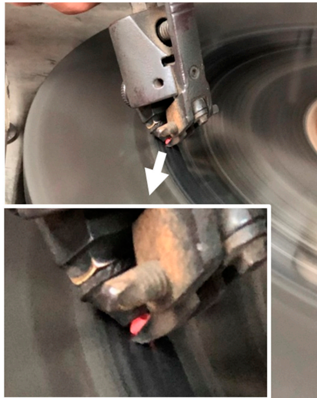
Figure 5. The polishing process of the rough diamond A (insert: the magnification of the “light emission by the heated diamond”).
