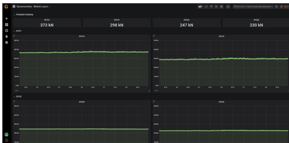
Figure 7. The Grafana system shows the loads on the gabion walls.
