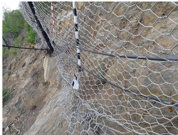
Figure 12. View of the second-generation accelerometer wireless sensor node in the plastic box with solar panel.
