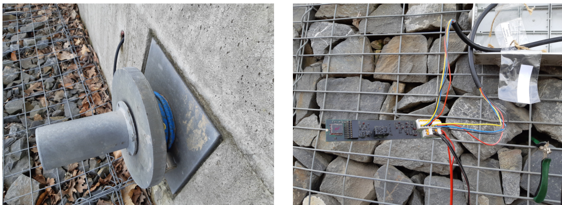
Figure 14. Load anchor cell sensor (left), load anchor cell wireless node outside the plastic tube (right).
