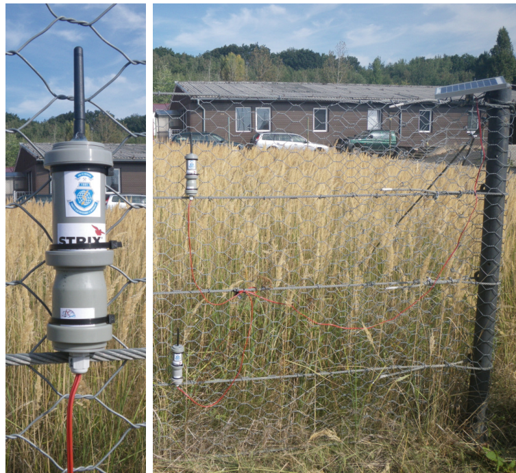
Figure 9. Detailed view of the accelerometer wireless sensor nodes in plastic tubes.
