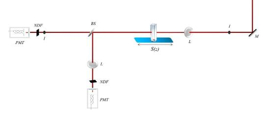
Figure 1. Configuration of the Z-scan technique.
