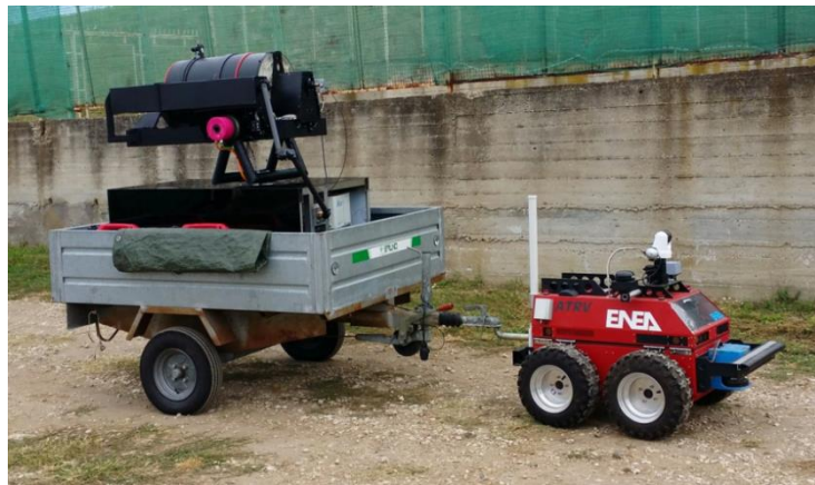
Figure 1. Integrated Laser Sensor (ILS) Prototype 2 placed on a trailer and driven by a remotely-operated vehicle.
