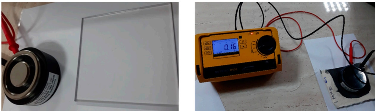
Figure 3. METRISO B530 Surface Resistance Tester and concentric ring probe 880.
