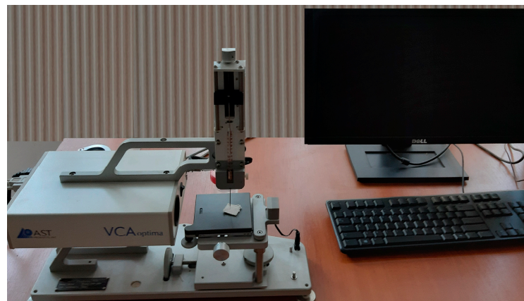
Figure 2. VCA Optima device for contact angle investigation (AST products).
