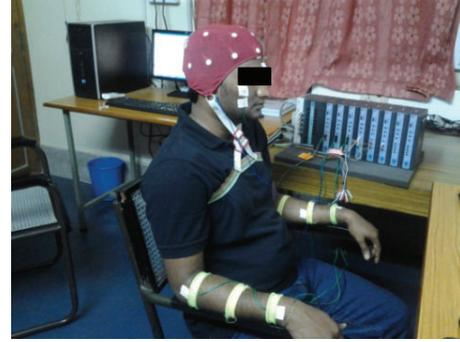
FIGURE 1: Recording setup for the BCI experiment.
