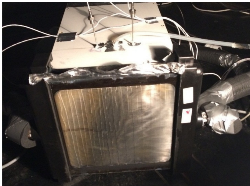
Figure 4. Front side of the heat exchanger connected to the entrance of the wind tunnel after injection of 200 g of the test dust.
