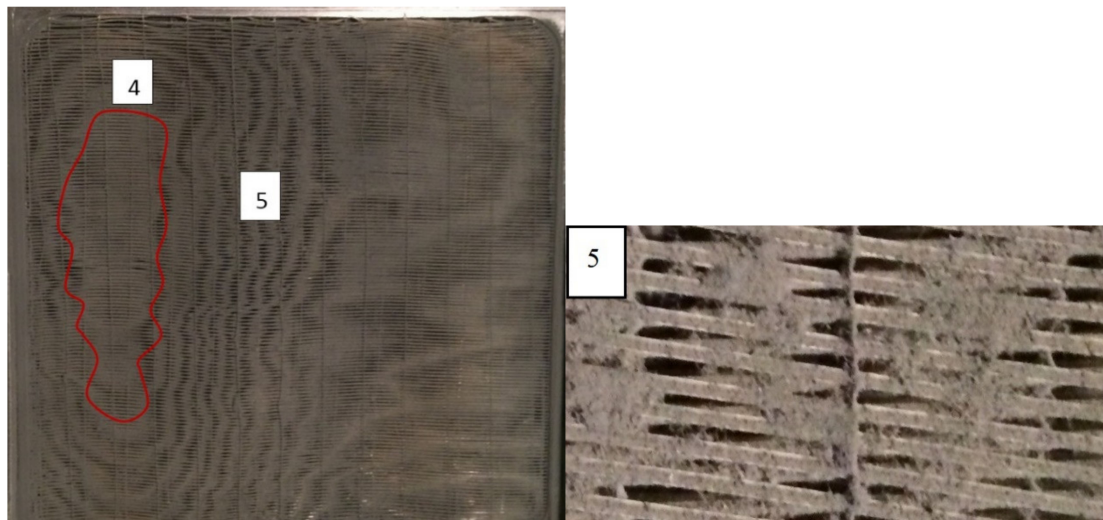
Figure 6. Heat exchanger surface after injection of 1200 \text{ g m}^{-2} of test dust (left). The majority of the front surface of fibers is covered with the deposit layer. There are zones where the deposit blocks the gap between the fibers (as in zone 4) or creates the lines of the blocked zones (as in zone 5, see details (right)).
