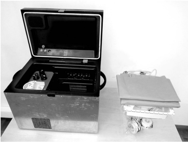
Figure 1. The heart preservation system. The size of the hardware is 55 \times 40 \times 44 cm and the weight is 26 kg (left). The disposable part (2.8 kg) is shown to the right. The heart is kept submerged in the preservation medium, making it insensitive to mechanical shocks and air emboli during transport. The system can be transported in regular airplanes, tolerating the angles that occur during take-off and landing.
