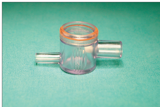
Fig. 1. The Epidrum ® is 2.5 × 2 cm in size and consists of a hard plastic body chamber, an injection port with a one way valve (right side), an outlet port to connect to the epidural needle (left side), and a soft, thin silicon membrane diaphragm on top of the device.
