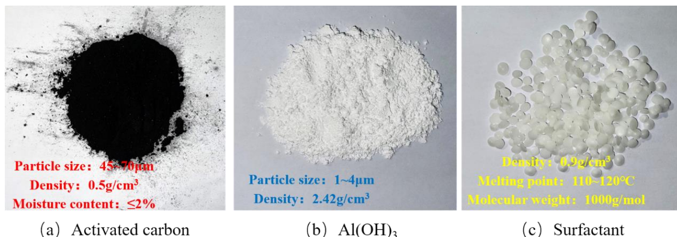
Figure 1. The schematics and properties of additives added for emission reduction; (a) Activated carbon, (b) \text{Al}(\text{OH})_3 , (c) Surfactant.
