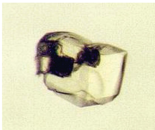
Figure 3 Photograph of a 400 \mu\text{m} neuraminidase crystal (subtype N9 from avian influenza isolated from a noddy tern), space group I432 , that has been irradiated on ID14-4 at the ESRF at 100 K and then allowed to warm up to RT. The three black marks are from the 100 \times 100 \mu\text{m} beam; the discolouration is an indication of radiation damage.
