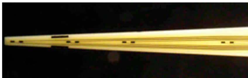
Figure 2. Detail of 8-TRK probe used in this project (CenMeT, University of Kentucky, Lexington, KY, USA). Each recording site is 50 \times 100 \mu\text{m} . Recording site pairs have 100 \mu\text{m} separation. The spacing between recording site pairs is 1 mm, 1 mm, and 2 mm [25].
