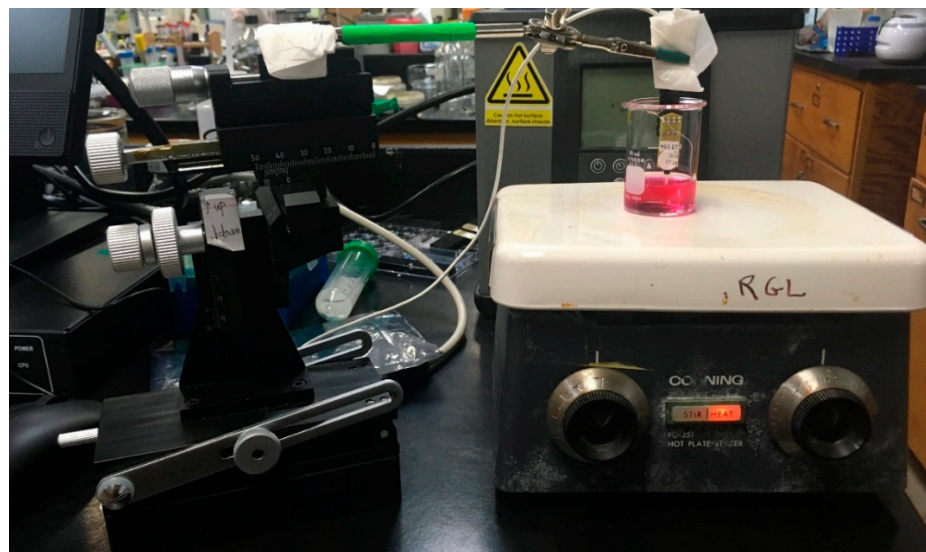
Figure 3. Experimental setup of the probe during calibration. The magnetic stirrer ensured a continuous steady flow of H 2 O 2 to the electrode surface.
