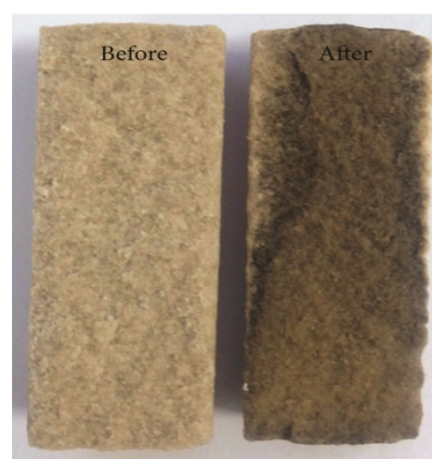
Figure 10. Image of the core profile before and after flooding [152].
