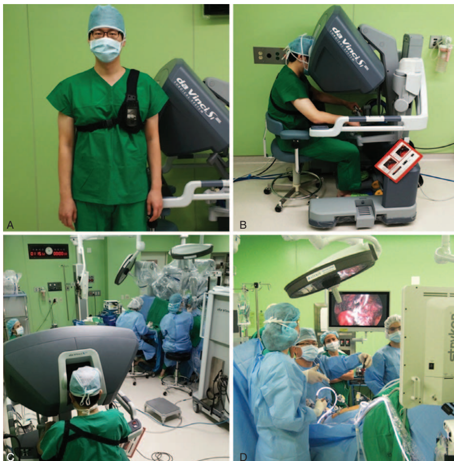
FIGURE 1. (A) The EMDEX Lite was fitted over each surgeon's heart during surgery. (B) The surgeon at the master console of the da Vinci Surgical System. (C) The operating table and surgeon during robotic surgery. (D) The operating table and surgeon during laparoscopic surgery.
