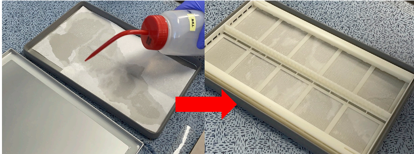
Figure 2. Setup of the humidity control tray in the HybEZ II hybridization system
