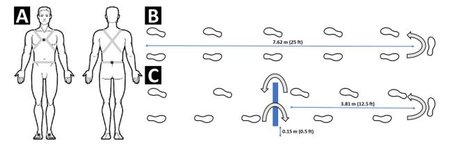
**Figure 1.** Inertial sensors placement (**A**) at the bilateral feet, chest, and lumbar spine and the sample courses for the walk and turn task (**B**) and walk and turn with obstacle task (**C**). For both tasks, the length of the course was 7.62 m (25 ft). The obstacle in the walk and turn with obstacle was placed at approximately 3.81 m (12.5 ft) from the starting position and was 0.15 m (0.5 ft) tall.
