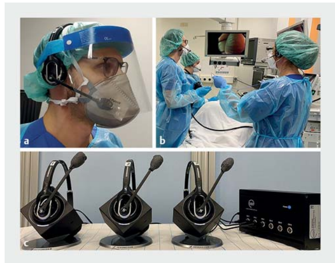
► Fig. 1 a DECT Intercom Headset with FFP3 and face shield in use for COVID-19 high-risk examinations. b Digital enhanced team communication within colonoscopy, endoscopist (left front), assisting nurse (right) and sedation performed by nurse (back left). PPE with FFP2 mask, hair net, gown and gloves for moderate risk stratification. c (Left) Cordless DECT Intercom Headsets with microphones on cubic charging station, noise-cancelling microphones equipped with disposable mike protector. (Right) Controller for connected audio communication (Intercom Box)
