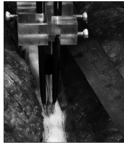
Figure 4: Process of coagulating a vessel on porcine spinal cord
