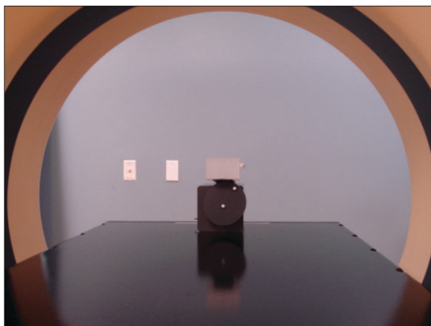
Figure 2: A modified motion phantom was used for time-delay measurement; the two plastic balls, on the axis and periphery, are visible
