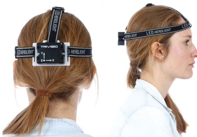
Fig. 1. Inertial microelectromechanical sensor fixed by a tight headband on a colleague's head.
