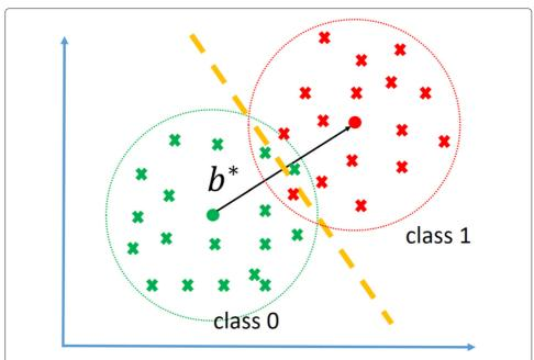
**Fig. 2** The illustration of the  $b^*$  selection process. Given V(X) vectors for the two classes, denoted by red and green crosses, the  $b^*$  is chosen to maximize the distance between the center of projections of V(X) vectors on b
