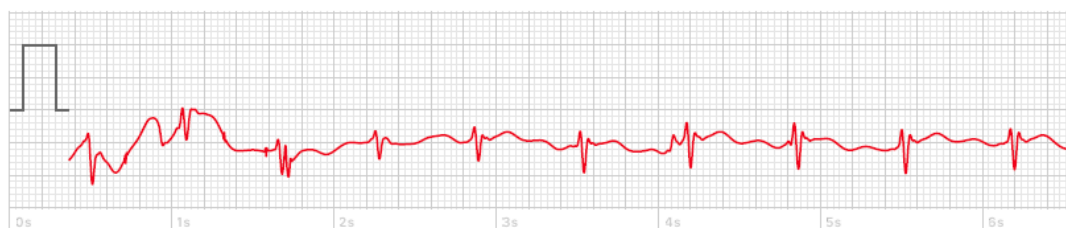
Figure 4. A sample of temporary artifact (around one second) due to instability of the Apple Watch 4 on a patient's wrist.
