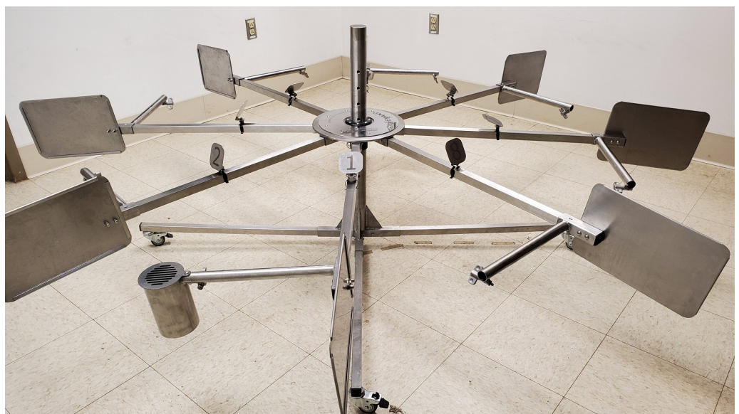
Fig 2. Photograph of the 8-port stainless-steel scent wheel used in this study (manufactured by DEMAND (design & manufacture for disability), Abbots Langley, UK, http://www.demand.org.uk ). Ports which held the odors moved between arms of the wheel for example, in "1" there is a port present—all other arms are empty.
