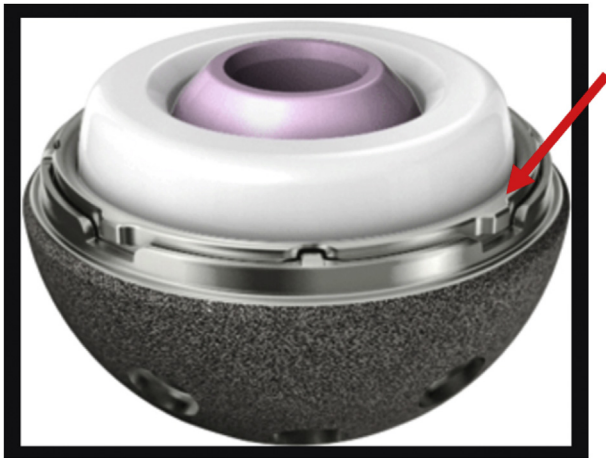
Figure 8. Stryker Orthopedics (Mahwah, NJ) modular dual mobility (MDM) hip system. Note the elevated acetabular insert (red arrow) that may be a source of femoral neck impingement, leading to micromotion at the modular surface and ultimately, mechanically assisted crevice corrosion (MACC).
