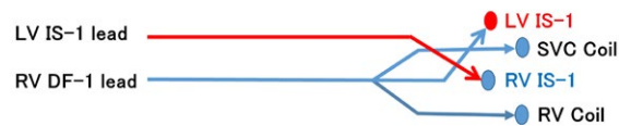
FIGURE 2 A, Left ventricular protection period. B, Troubleshooting of this case. LV lead was plugged to the RV IS-1 port and vice versa (RV IS-1 to the LV IS-1 port)
