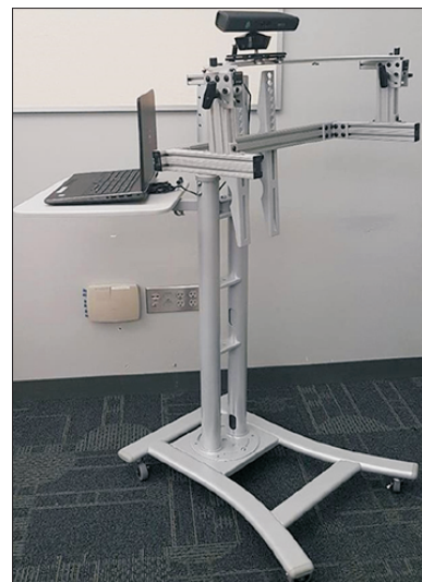
Fig. 2. The Pectus Metric Tool 3-dimensional body scanner using Microsoft Kinect.
