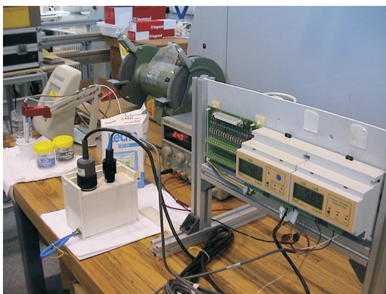
Figure 5. Off-line testbed for evaluation of probes. At rear is the laboratory EC probe and in front are C1 and C2 probes inserted at one measurement chamber.
