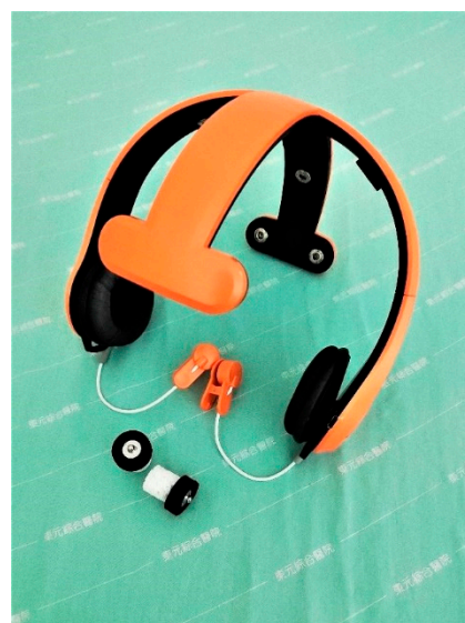
Figure 3. Wireless EEG device. A wireless and wearable EEG headset ( top ) and novel hygroscopic sponge electrodes ( bottom ). The sensors can be easily and quickly assembled, and fit appropriately into the original device.
