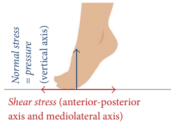
FIGURE 2: Normal stress (pressure) is vertical axis. Shear stress is the resultant force of anterior-posterior axis and mediolateral axis.
