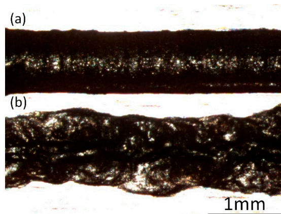
Figure 14. Channel morphologies under the VG of 400 μm at: (a) 0.1 mm/s; and (b) 0.2 mm/s.
