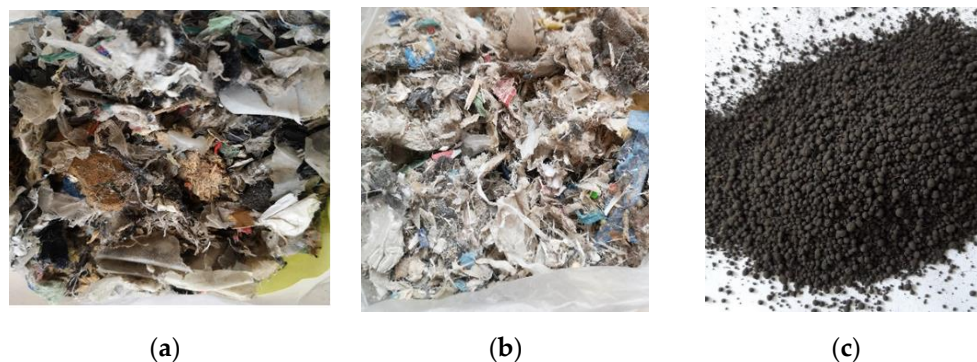
Figure 2. The tested waste sample: (a) refuse-derived fuels–RDF 1, (b) refuse-derived fuels–RDF 2, and (c) sewage sludge–SS.
