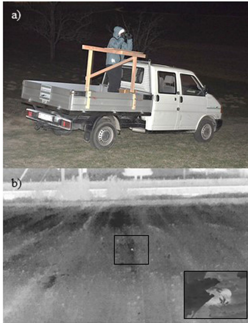
Figure 1. (a) Setup for the application of the handheld thermal camera. (b) Suspicious thermal signature in a distance of about 40 meters, corresponding to a leveret in terms of size, shape and brightness. Identification is not possible, thus close inspection is necessary. Small picture: close-up of a thermal signature of a leveret from a distance of 3 meters. Both pictures have been captured with a handheld FLIR Scout TS-32r Pro thermal camera.
