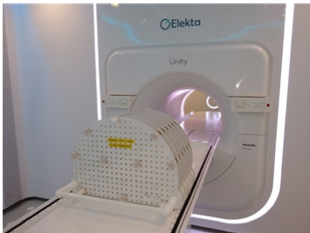
FIG. 3. Geometric distortion phantom supplied with the Elekta Unity MRI-linac.
