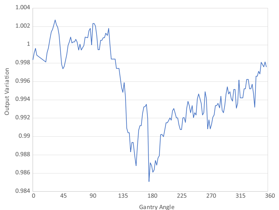
Fig. 8. Angle-Dependent Cryostat Attenuation Map. All results are normalized to the results measured at a gantry angle of 90°.
