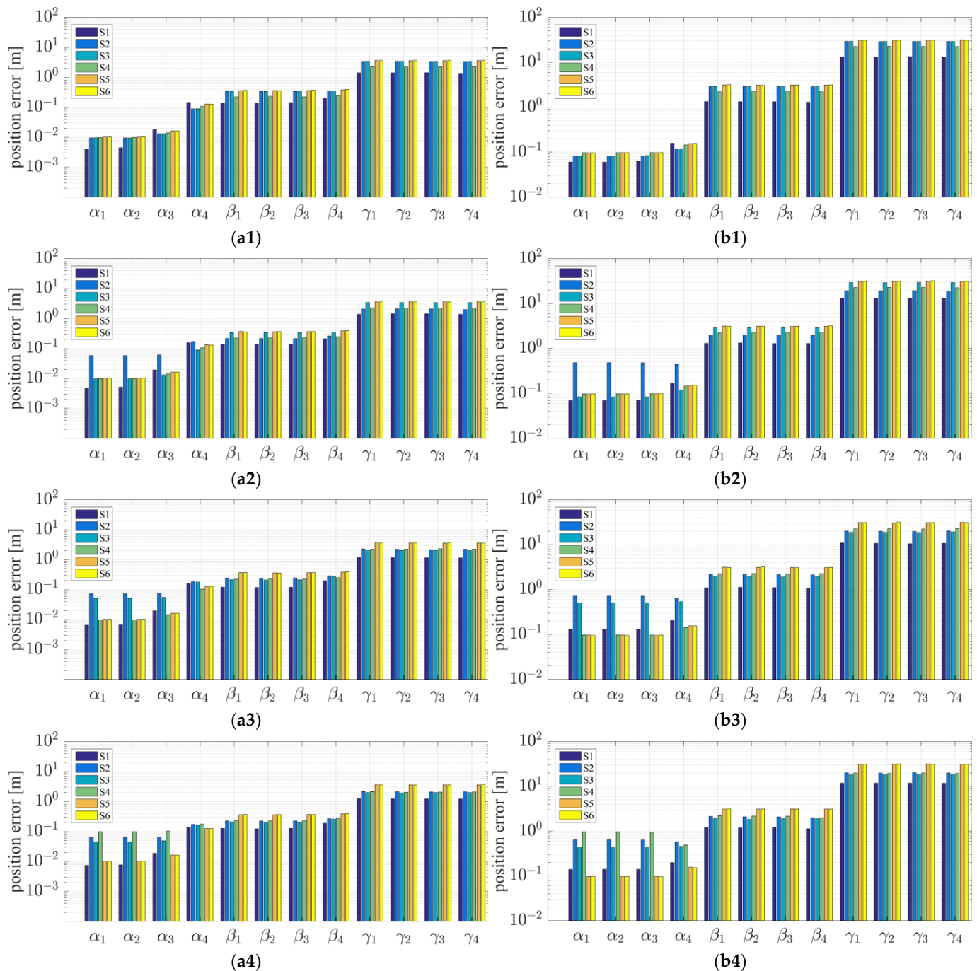
Figure 18. Statistics on the relative navigation accuracy under different simulation scenarios: (a1) Case a: space-circle radius 1 km and 6 chief satellites; (b1) Case a: space-circle radius 10 km and 6 chief satellites; (a2) Case b: space-circle radius 1 km and 5 chief satellites; (b2) Case b: space-circle radius 10 km and 5 chief satellites; (a3) Case c: space-circle radius 1 km and 4 chief satellites; (b3) Case c: space-circle radius 10 km and 4 chief satellites; (a4) Case d: space-circle radius 1 km and 3 chief satellites; (b4) Case d: space-circle radius 10 km and 3 chief satellites.
