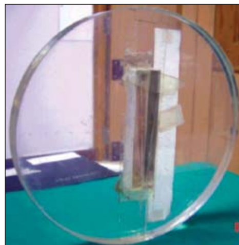
Figure 1: In-house fabricated sensitivity profile phantom
