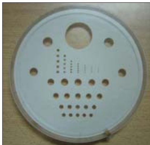
Figure 2: In-house fabricated low-contrast resolution phantom
