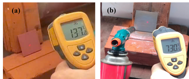
Figure 6. Paint samples G-0.05 were heated with shock (a) when the surface sample reached 137 °C and (b) after 30 min reached the highest temperatures of 730 °C.
