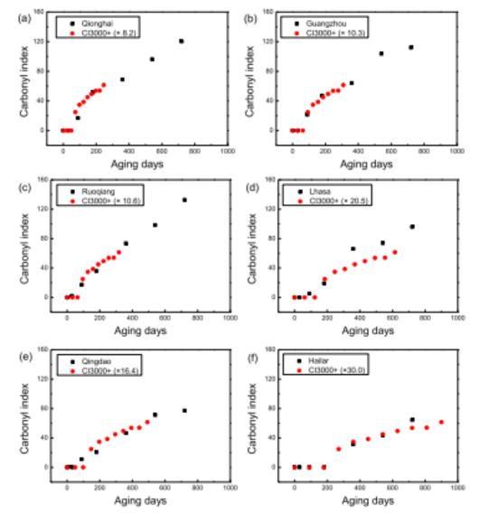
**Figure 4.** Comparison between results from outdoor exposure, performed in six different locations in China ((**a**): Qionghai; (**b**): Guangzhou; (**c**): Ruoqiang; (**d**): Lhasa; (**e**): Qingdao; (**f**): Hailar), and predictions from accelerated aging, based on carbonyl index. Reprinted with permission [31].
