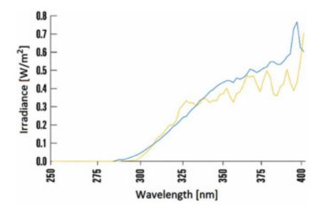
**Figure 2.** Comparison between the characteristic radiation spectrum of the xenon lamp (with a filter approximating the spectrum of sunlight), blue line; and the spectrum of sunlight, yellow line. Reprinted with permission [19].
