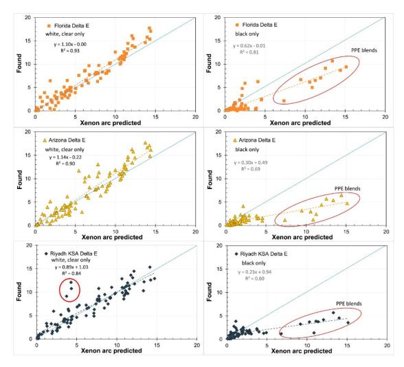
**Figure 5.** Found vs. predicted color shifts for white and clear materials (**left**) and black materials (**right**). The blue dotted lines show slope = 1 while the colored dashed lines show the linear regression with the equation in the legends. The three circled points on the lower left plot occurred near an abrupt color shift. The circled points on the right side graphs show the PPE blends. Reprinted with permission [18].
