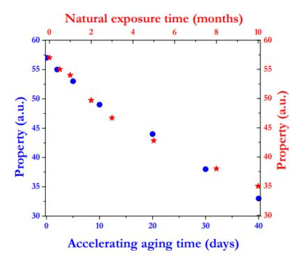
**Figure 3.** Correlation between the values of an arbitrary property measured on a polymer outdoor exposed and those recorded for the same polymer subjected to an accelerated aging procedure, with the aim to calculate an "Equivalent time".
